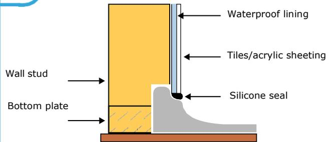
These bases are designed to be installed in a stud wall. Make sure there is clearance between the base's tile lip and the wall stud to allow for any movement.
