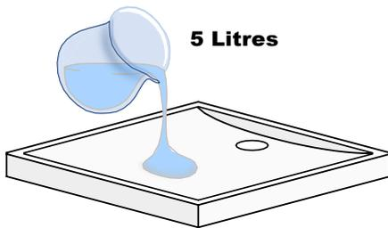
Put base on a level surface and water test with 5 litres of water to ensure it drains correctly. If this is not possible, a small spherical object placed in each corner will suffice.
